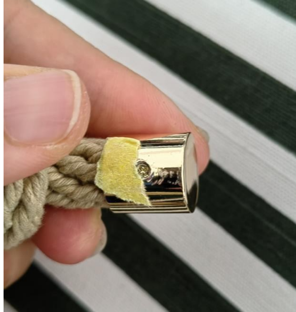
027- defect-metal scratch on surface
