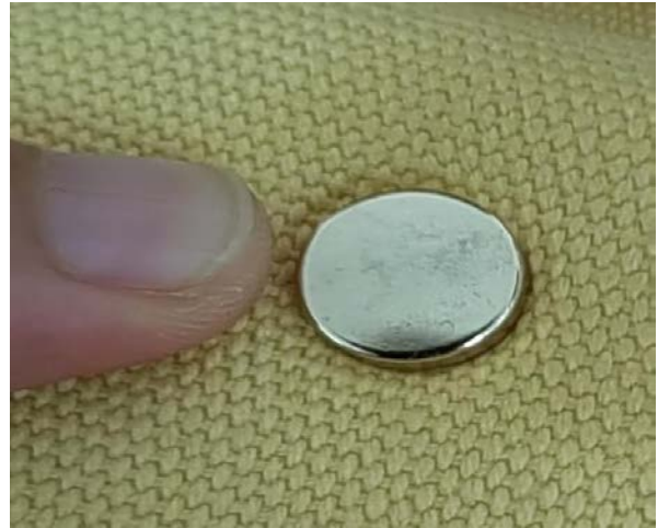
032- defect-scratch on surface
