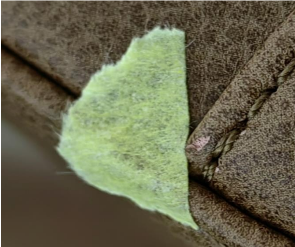
025-defect-pu damage on surface
