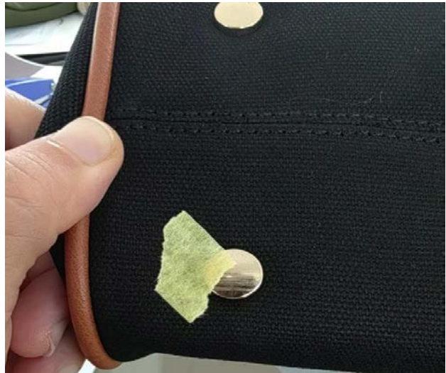
028- defect-metal scratch on surface
