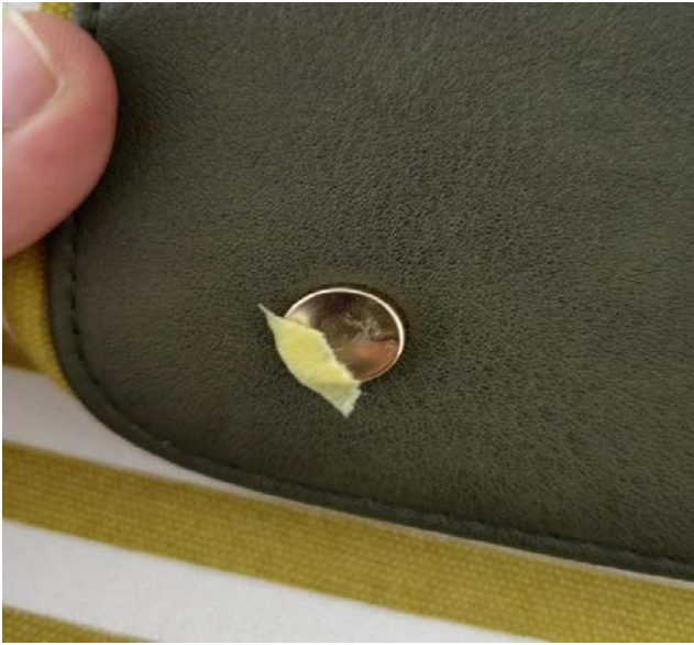
024- defect-metal scratch on surface
