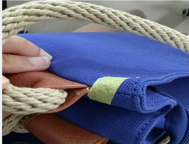
031 - defect-PU damaged on surface
