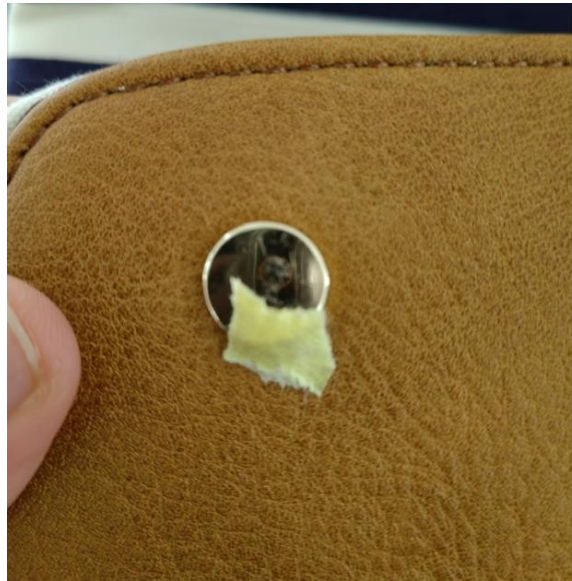
025- defect-metal scratch on surface
