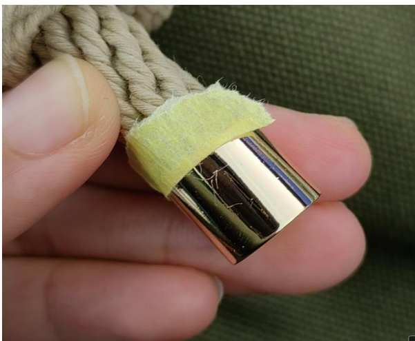
029 - defect-metal scratch on surface-major
