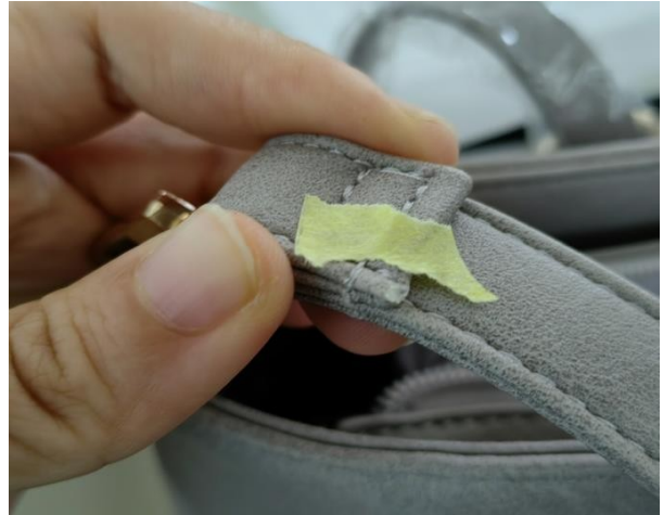
026-defect-pu damage on surface
